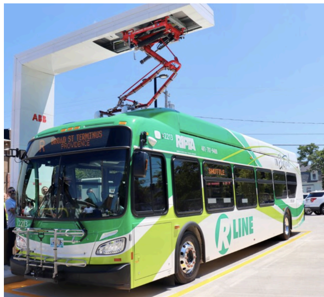
Figure 7: Existing overhead charging station in Providence, Rhode Island to charge the state's first fleet of battery electric buses (Reed, 2024)
